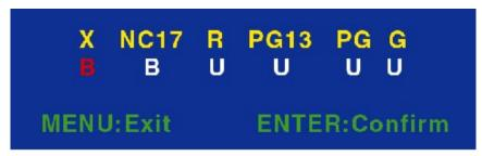
Select MPAA Rating Guide to set rating grade. Use remote control arrow keys to move cursor to desire rating grade. When the text turns red, press ENTER key to set block (B) or unblock (U) condition.
